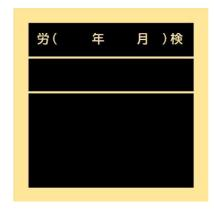
According to Japanese regulations, each certified equipment must be affixed with a certification label in addition to Ex marking label. The label needs to be as specified by the regulation as described below:
